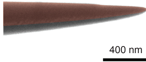
Figure 2.6.1: Scanning electron micrograph of a quartz tip with magnetic coating. The metal coating is overlain in red (false color).
