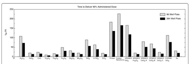
Figure 3 Comparison of time required to deliver 90% of the administered dose ( $t_{90}$ ) in hours (h), calculated following the described dosimetry methodology, for all materials investigated in two well plate configurations.
