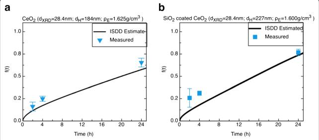
**Figure 2 Validation of dosimetry methodology for two metal oxide ENMs. a.** Validation of dosimetry approach for CeO<sub>2</sub> (d<sub>XRD</sub>=28.4 nm) suspended in DMEM; **b.** Validation of dosimetry approach for SiO<sub>2</sub> coated CeO<sub>2</sub> (d<sub>XRD</sub>=28.4 nm) suspended in DMEM. All experiments were done in triplicate, error bars represent standard deviation.
