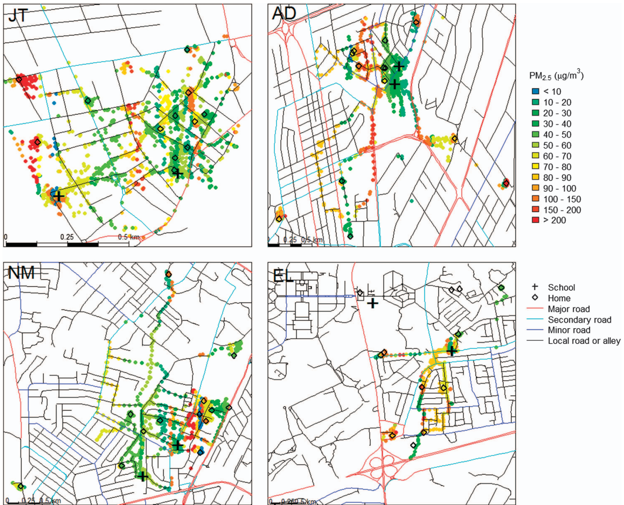
Figure 3. Spatial pattern of PM_{2.5} exposures of the study subjects, by neighborhood. The graph shows average of all minute-by-minute exposures, with averaging done in 20\text{ m} \times 20\text{ m} grids. Annual geometric mean PM_{2.5} concentrations at residential monitoring sites were 50.5\ \mu\text{g}/\text{m}^3 in JT, 31.1\ \mu\text{g}/\text{m}^3 in AD, 28.4\ \mu\text{g}/\text{m}^3 in NM, and 23.2\ \mu\text{g}/\text{m}^3 in EL. Annual geometric mean PM_{2.5} concentration at a roadside monitoring site was 35.2\ \mu\text{g}/\text{m}^3 in NM. 4
