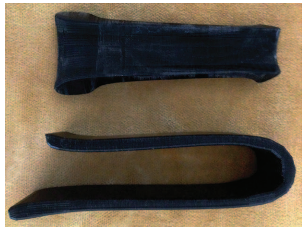
Fig. 3. Splints printed by FDM. Material used: acrylonitrile butadiene styrene. Cost: 5 cents per gram.
