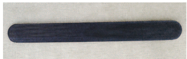
Fig. 4. Tongue depressor printed by FDM. Material used: acrylonitrile butadiene styrene. Cost: 5 cents per gram.
