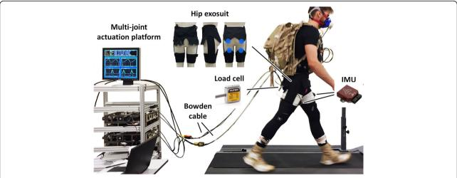
**Fig. 1** Experimental setup with a participant wearing a soft exosuit that assists hip extension via Bowden cable. The assistive force is transmitted from the multi-joint actuation platform (on the left) to the wearer
