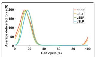
**Fig. 2** The resulting assistive force profiles with SEM (average from eight subjects) are shown on the right side of the figure. Early-startearly-peak (ESEP), early-start-late-peak (ESLP), late-start-early-peak (LSEP), late-start-late-peak (LSLP) in red, yellow, green, blue respectively
