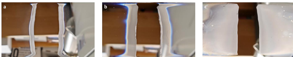
Figure 4-25: (a-c) Optical images of three \text{SnBr}_2 depositions with (b) deposited at a hotter temperature than (a), and (c) deposited at a hotter temperature than (b). These images agree with the spreading of the deposition width as shown in Figure 4-24.
