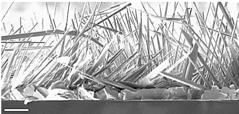
Figure 4-12: SEM cross-sectional image of a \text{SnBr}_2 “forest” deposited at 160 °C for 20 min with \text{Sn}(\text{hfac})_2 at a source bubbler temperature of 65 °C. The accelerating voltage was 3 keV at a working distance of 7 mm. The scale bar is 10 \mu\text{m} .
