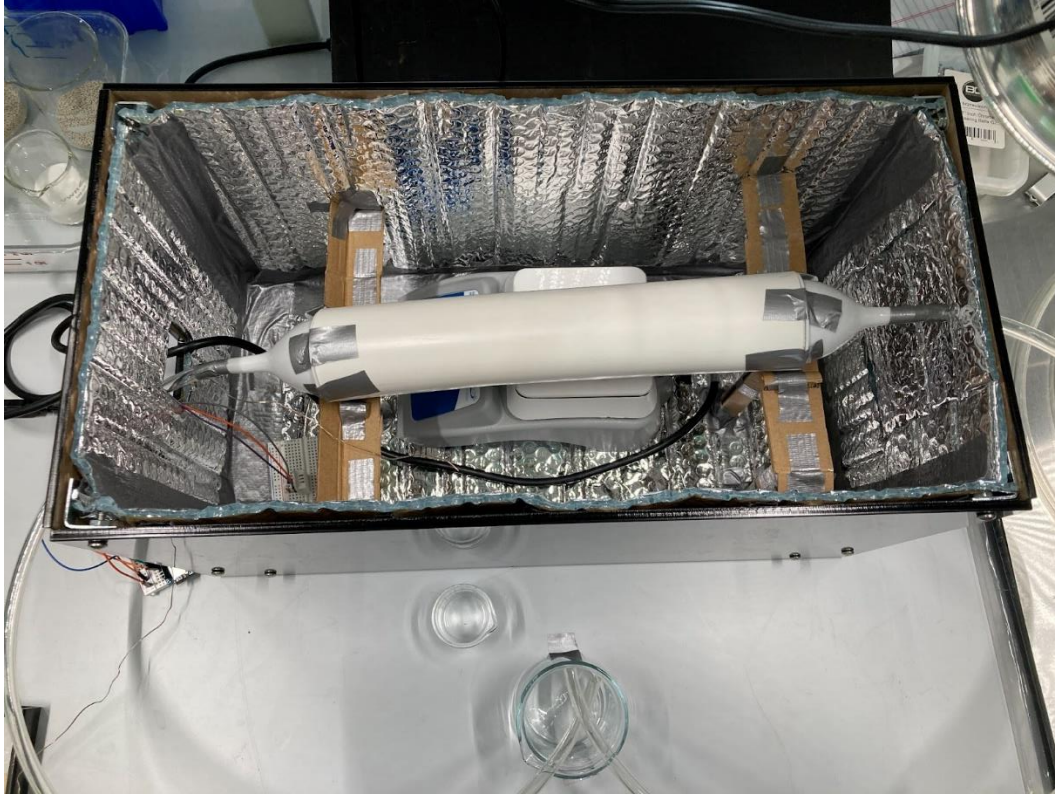
Figure 12 - Image of device interior components as initially assembled. This includes the suspended PVC pipe to hold sorbent materials, funnels and tubing to collect water during the desorption cycle, the exterior final collection site, a sensor, and a hot plate. Some minor changes were later made to this build based on test results, such as changing tape connections to Velcro tape and switching from one collection site to two.
