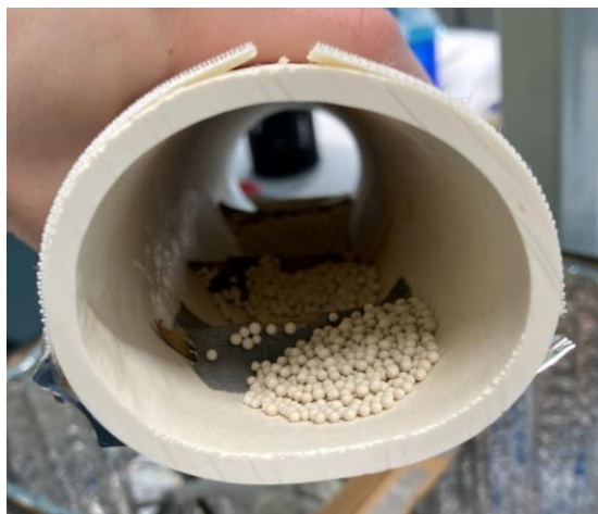
Figure 11 – Image of PVC pipe interior, showing several ridges along the length to hold sorbents in place while pipe is sloped. Zeolite 3A has been added to the pipe in this image, although due to a slight rotation while taking the image, some of the material has moved slightly. It would be spread out more to maximize surface area for absorption during operation of the device.
