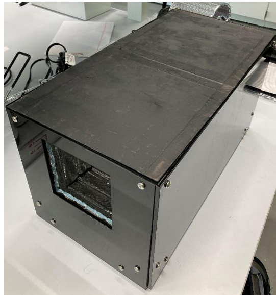
Figure 10 - Built Device Exterior Structure. Exterior hard plastic walls have been assembled, along with the solar thermal absorber including insulation and black aluminum sheet. At this stage, the interior components are not yet present.
