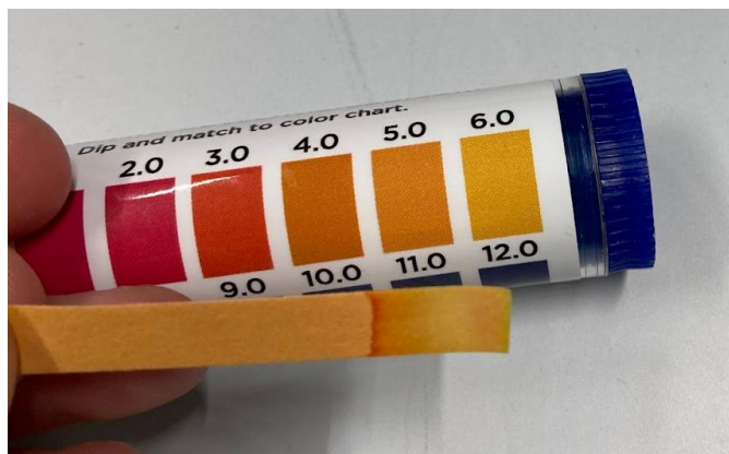
Figure 21 - Image of pH testing strip results from Trial 1. In each trial the results were closest to a pH of 6, which is relatively close to the EPA standard range of 6.5-8.5 when considering the lack of precision.
