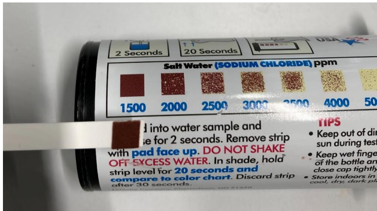
Figure 22 - Image of sodium chloride testing strip results from trial 1. In each trial the results showed a level of 1500 ppm or less, the lowest possible with the strips used. This low value means that sodium chloride, and by proxy conductivity, should not present any water quality issues.
