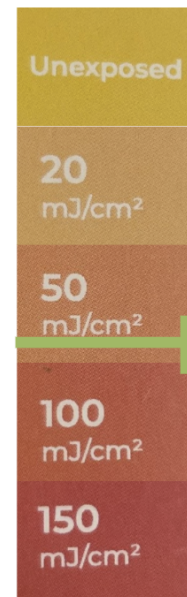
(b) UVC Dosimeter Color Scale
