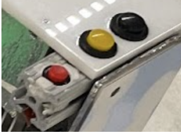
Figure 6.14: From Left to Right: Power Shut Off Button, Program Start Button, and Reset Button
