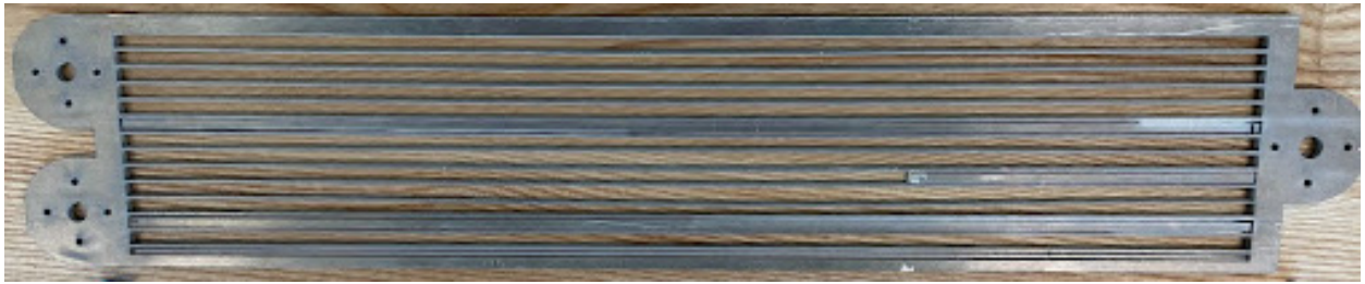
Figure 6.6: Waterjet Cut Scale Initial Prototype of the Moving Platform
