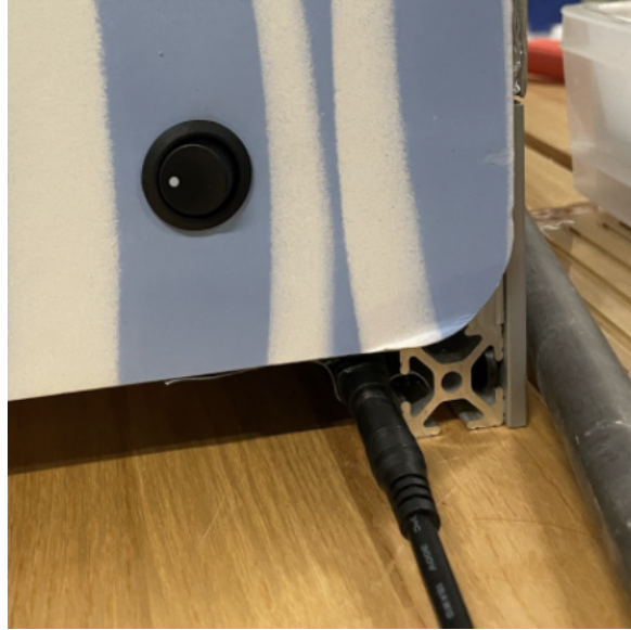
Figure 6.11: Input from Wall Plug and Power Switch on the Front of the Device
