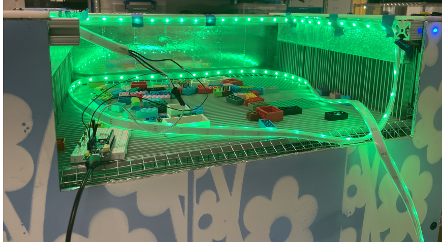
Figure 8.1: LED Testing Setup within the Device
