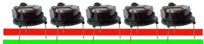
Figure 6. A visualization of the Kilobot charging scheme.
