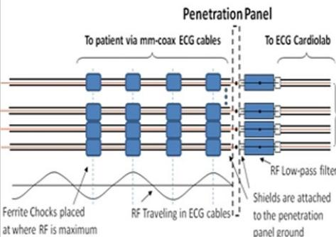
Fig.3: GR-RF blanking circuit for selective EAM signal acquisition (response time<200ns)
