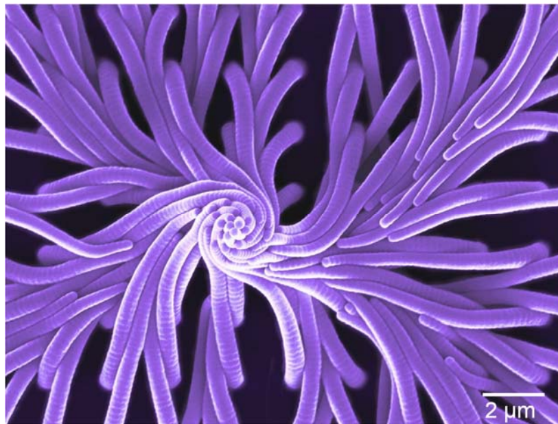
Figure 2. An image of a single fiber arrays shown in Fig. 1 self-organized into a complex pattern by interaction with an evaporating liquid. The image was taken with a SEM and was digitally enhanced for color. Reprinted from ref. 2 with permission from AAAS.
