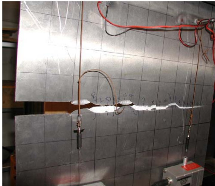
Figure 2: A 10mm thick plate of A5083 aluminum tested by Simosen and Törnqvist [5]. The crack was initiated at the edge notch located on the left edge of the plate. Flipping of the slant fracture from one 45 degree orientation to the other is evident.
