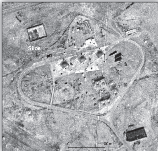
Figure 2 (below). Figure 2. GAMBIT photograph of subterranean ICBM silos at Baikonur, Kazakhstan (Mission 4033, 13 October 1966). The three silos at center have domed covers that slid on rails to the left before launch.
