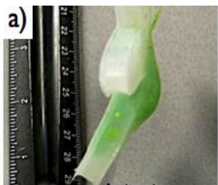
Figure S5. Photos of the hydraulic actuation of an elastomeric gripper and its puncture and self-sealing. a) non-actuated gripper, b) actuated gripper, c) puncturing the inflated side of the gripper with 3.76 mm diameter nail, d) punctured gripper maintains actuation, e) gripper still functions after the nail is removed.
