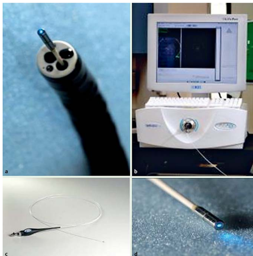
Fig. 1 The probe-based confocal laser endoscopy (pCLE) system. a Probe within standard endoscope. b Laser scanning unit and display. c Fiber probe. d Fiber probe with blue laser illuminated.
