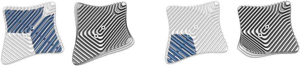
▲ Figure 16: Chamber location and deformation. Left: Chamber A. Right: Chamber B.
