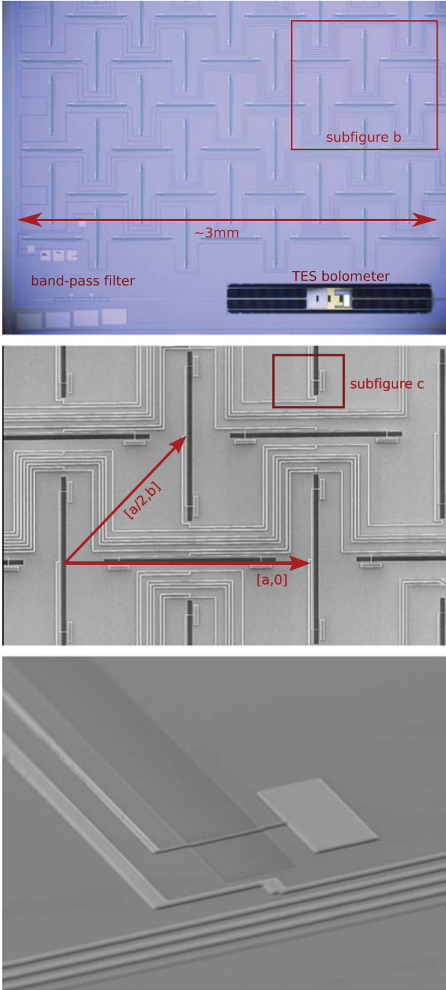
Figure 2. Optical and SEM photographs of major features of the antenna array. Upper: one quarter of a detector element. The antenna array, one filter, and one TES bolometer are visible, as well as DC readout lines for the detector. Middle: SEM micrograph of the slot array (dark rectangles) and oblique Bravais lattice (arrows). The thin white lines comprise the microstrip feed. For 150 GHz detectors, a \sim 600 \mu\text{m} and b = a/2 \sim 300 \mu\text{m} ; the slot dimensions and spacing in the 95 GHz are 63% larger and those in the 230 GHz detector elements are 47% smaller. Lower: SEM micrograph of microstrip crossover and shunt capacitor at a sub-antenna slot.
