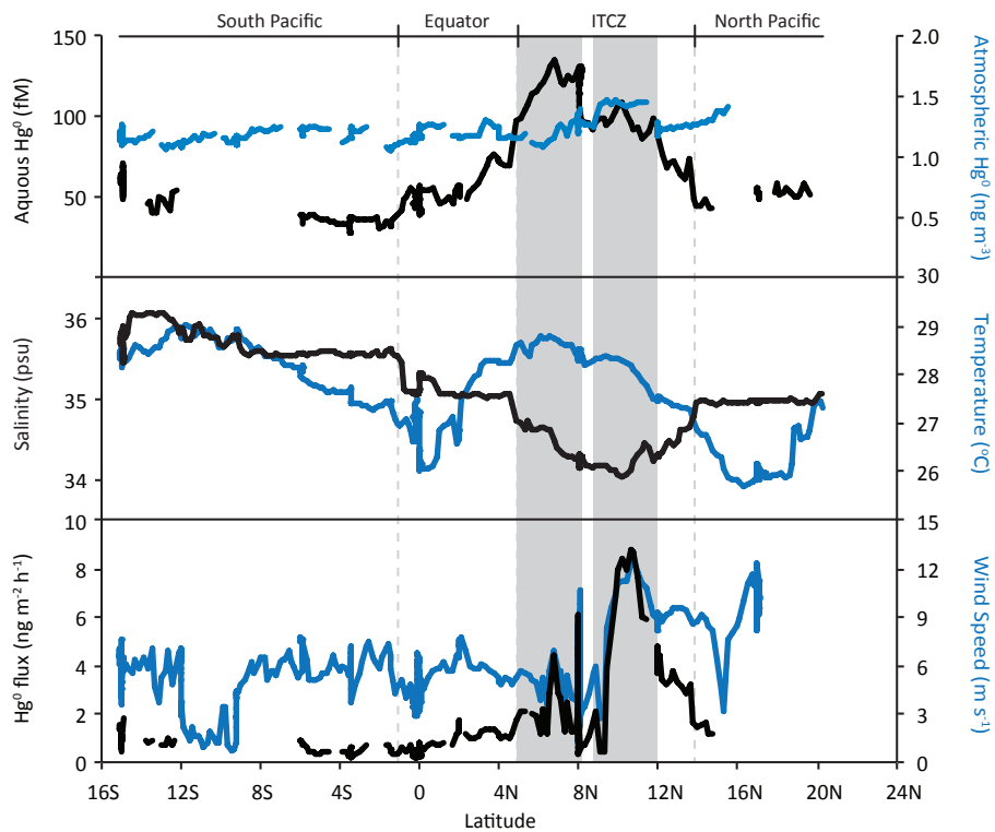
Figure 1. Latitudinal variability in measured atmospheric and seawater Hg 0 concentrations, associated evasion, and environmental properties on the METZYME cruise between 1-24 October, 2011. Oceanographic regimes for October 2011 are shown; shaded areas denote statistically different regions for Hg 0 concentrations within the oceanic regime reflecting the ITCZ.
