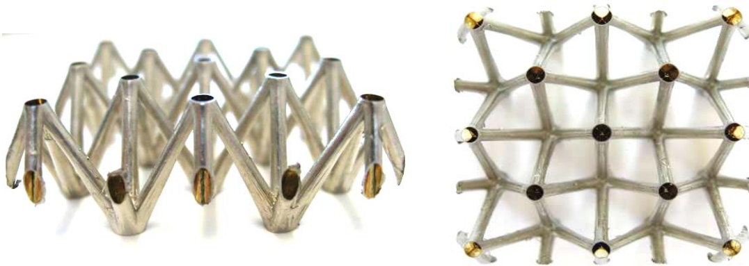
Figure 2 (a). An image of an HRL micro-lattice. (b) An image of a hollow truss Ni micro-lattice.
