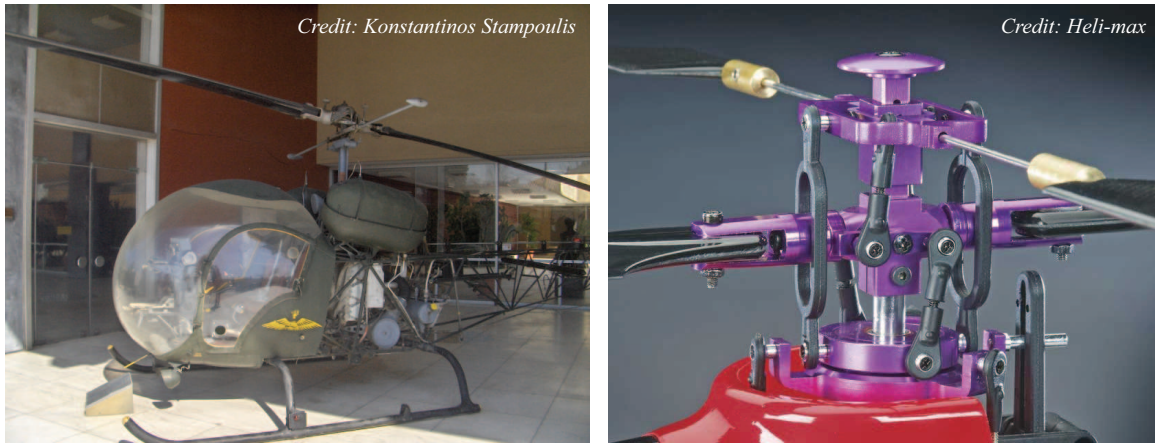
Figure 2.3: (left) The Bell Sioux H-13, incorporating a stabilizer bar. (right) A Heli-max Axe CPv3 radio controlled helicopter incorporating a Bell-Hiller stabilizer.
