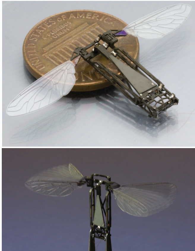
Figure 4.34: A completed Mobe (top) on a US penny and a composite image (bot) demonstrating flapping motion under an applied sinusoidal voltage to the piezoelectric actuator.
