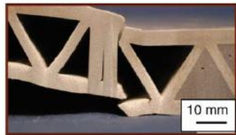
(c) Panel edge failure
