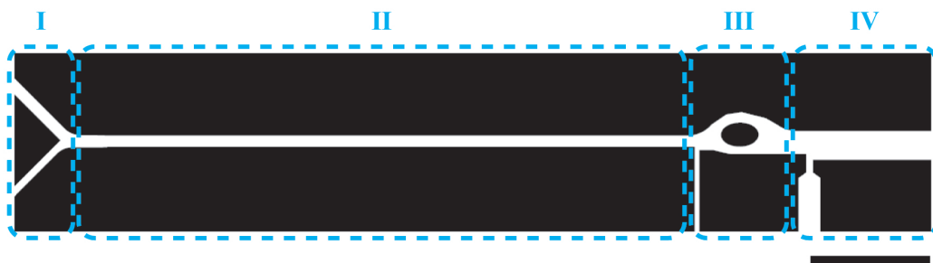
Figure 4.9: Schematic of the microfluidic device for coalescence of droplet pairs by addition of fluorinated alcohol. Droplet pairing occurs in region I, and the pair are brought together and steered toward the bottom wall in region II. Fluorinated alcohol is added to the continuous phase in region III and the droplets coalesce. The coalesced droplets are restabilized by dilution of the alcohol and the addition of fresh surfactant in region IV. Scale bar represents 500\ \mu\text{m} .
