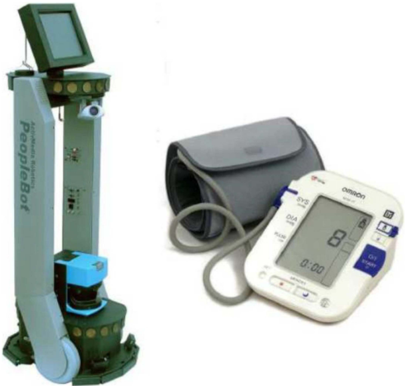
Figure 1. Peoplebot robot and blood pressure monitor that was attached to it for the study. doi:10.1371/journal.pone.0072589.g001
