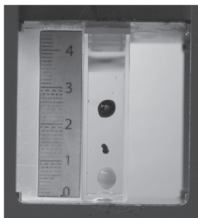
Figure 4. (a) A sample of gunpowder (Hercules Blue Dot) was levitated in a cuvette containing a 4.0M MnCl 2 solution and two density standards (1.450 and 1.800 g/cm 3 ; dark and light color, respectively) was placed in the MagLev device and a photo taken after 360 seconds. (b) The levitation height and corresponding density values for each gunpowder sample analyzed. The reported values are from seven independent measurements, with each measurement containing 3 pieces of gunpowder.
