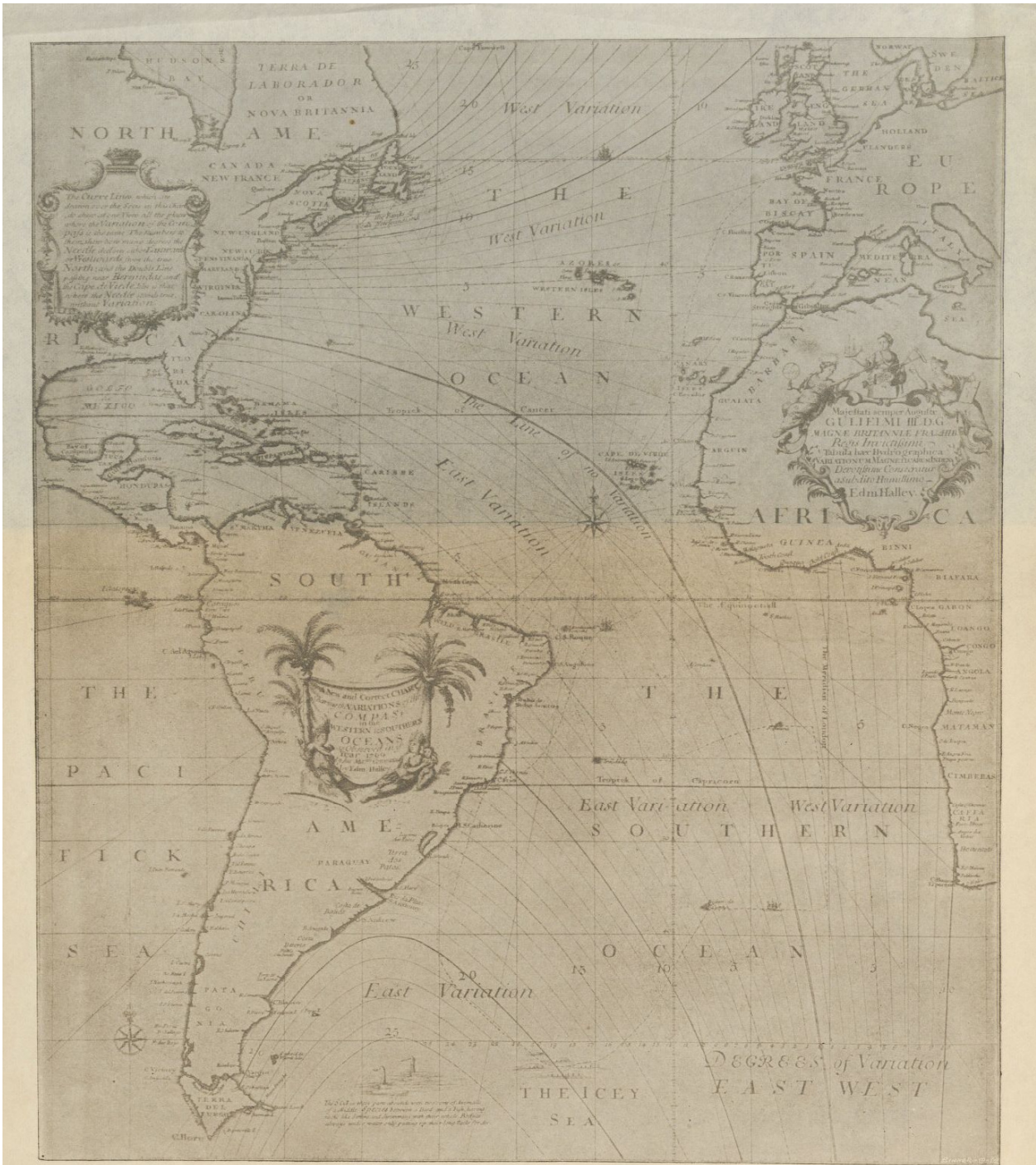
Figure 1.7: Edmond Halley’s Isogonic Chart showing lines of equal magnetic variation for the year 1700. 58
