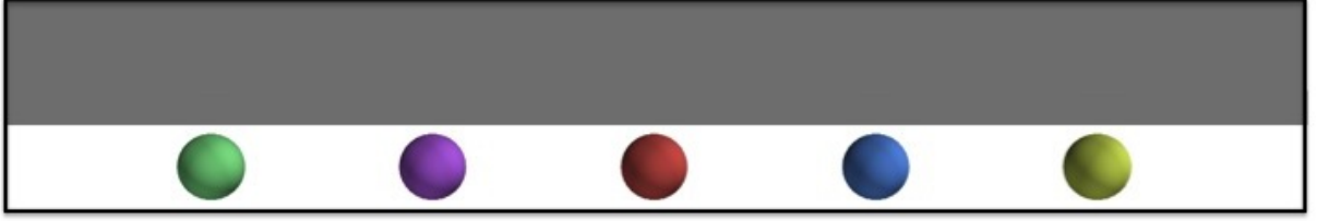
Figure 5.5: Zero bond local minimum. There are N!/2 ways to arrange the beads on the stripe, each of which corresponds to a basin in the energy landscape. For high N , most of these arrangements have very few ( \leq 2 ) bonds along the chain (but each arrangement has all N particles bound to the stripe). Here is an arrangement of 5 spheres lacking any bonds along the chain.
