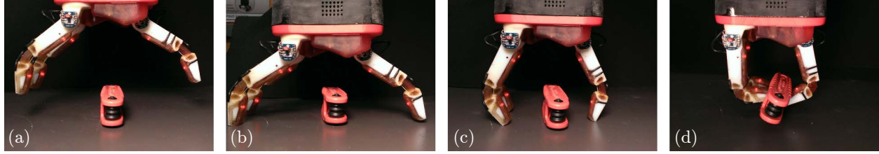
Figure 6.8: The surface grasp consists of (a) orienting the hand over the object, (b) performing a guarded move towards the surface, (c) slowly lifting the arm while the fingers maintain contact with the surface until the object is detected by the change of finger closure rate, and (d) tightening of the grasp for a firm hold.
