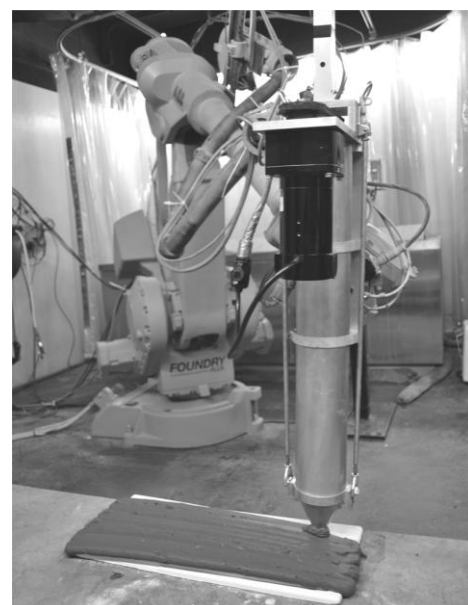
Fig. 7 Ceramic deposition in progress
