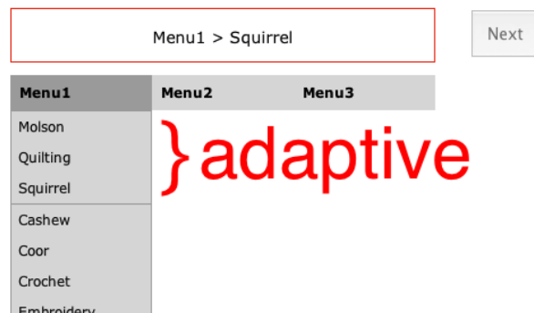
Figure 1: Split Menu. The three most recently selected items are copied in the adaptive top part of the menu.
