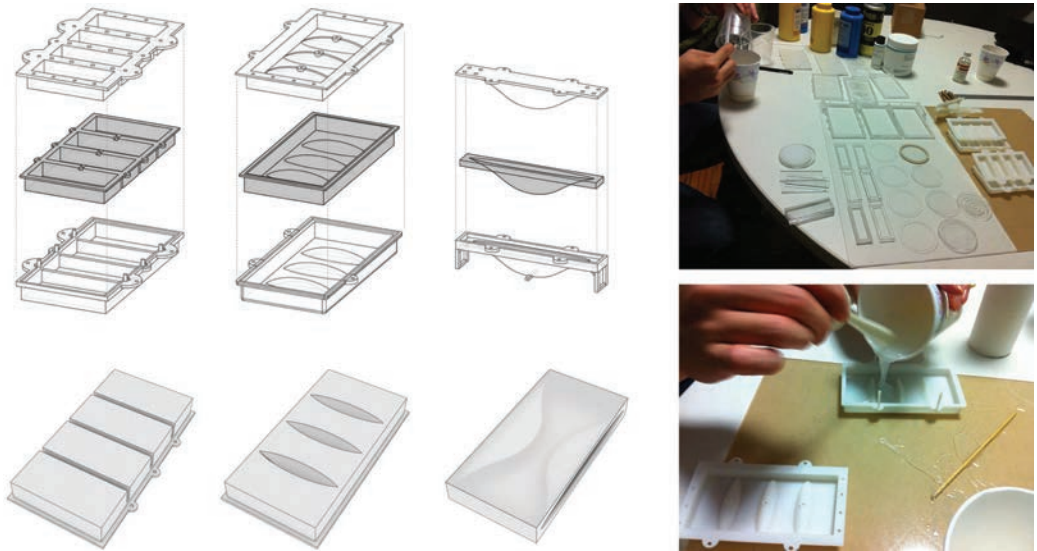
► Figure 18: Second stage mold and cast geometry and casting process.
