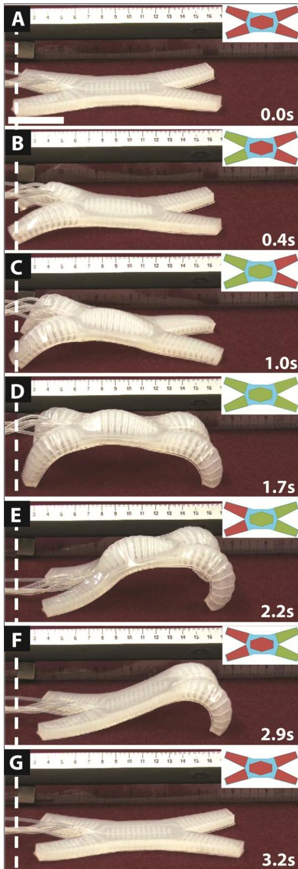
**Fig. 3.** (*A-F*) Cycle of pressurization and depressurization of pneu-nets that results in crawling. The particular pneu-net(s) pressurized in each step are shown (insets) as green, and inactive pneu-net(s) are shown (insets) as red. The scale bar in *A* is 4 cm.
