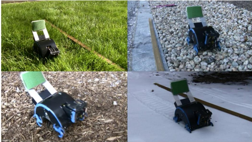
Figure 4.8.a. Exploiting whegs, the robot is able to traverse various surfaces with simple control.
