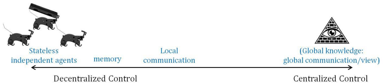
Figure 3.3.a. Sliding scale of knowledge, from an omnipresent centralized controller to a decentralized system with completely independent agents. Agent knowledge may be increased by exploiting memory and communication.
