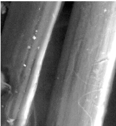
Figure 5. Modern specimen of Antheraea mylitta showing distinctive longitudinal striations in fibroin brins. Photomicrograph by I. Good and M. Derrick.
