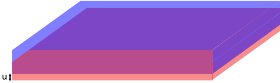
Figure 3.1: A simplified model to explain the formation of Volume Plasmon. The red cloud corresponds to the fixed ion cloud and the blue cloud corresponds to the electron cloud. The electron cloud is displaced from the positively charged ion cloud by a distance of u .
