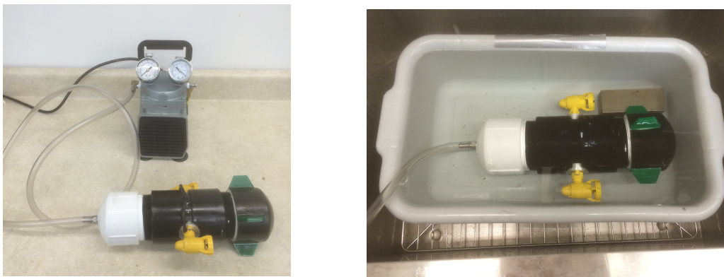
Figure 22: (left) Vehicle attached to air compressor, (right) Vehicle submerged to detect any air escaping
