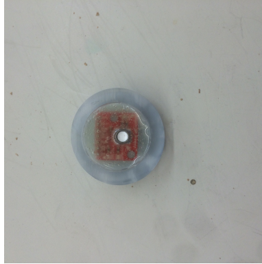
Figure 5: MS5803 -14BA pressure sensor in waterproofed housing
