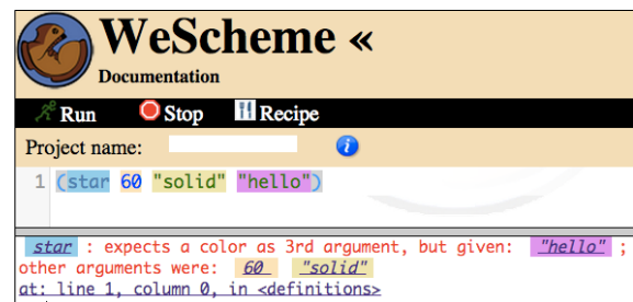
Figure 13 - A structured error message in WeScheme. Note the use of color and readable language.
