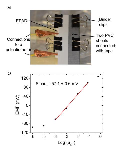
(dynamic) range of the paper devices (10<sup>-4</sup> to 10<sup>-1</sup> M) is comparable to that of the conventionally assembled device (~10<sup>-5</sup> to 10<sup>-1</sup> M, Figure S5a); this observation indicates the wax-printed paper layers and the paper reference electrode function as well as the plastic/glass electrode bodies used in commercial reference electrodes.
