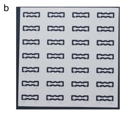
The ion-sensing EPADs are fabricated in a planar structure, and are thus appropriate for mass fabrication. As shown in Figure 1b, one page of chromatography paper (Whatman 1 Chr, 20 cm by 20 cm) can be used to fabricate 28 devices. It takes less than 30 minutes to fabricate one page of EPADs manually (28 or more devices, depending on the device configuration; *vide infra*). The efficiency of fabrication would be greatly improved by machine-based roll-to-roll printing.
