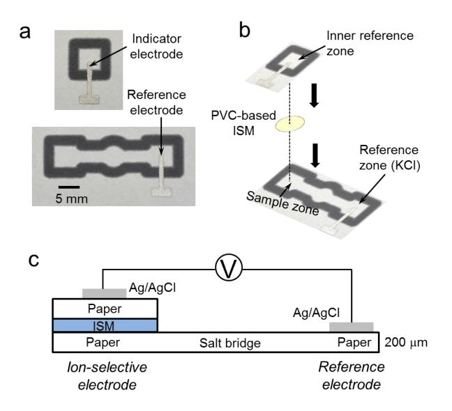
perform functions similar to those of their conventional counterparts. Analogously, paper components in the ion-sensing EPADs for K<sup>+</sup>, Na<sup>+</sup>, and Ca<sup>2+</sup> can also be mass fabricated (Figure S3).
