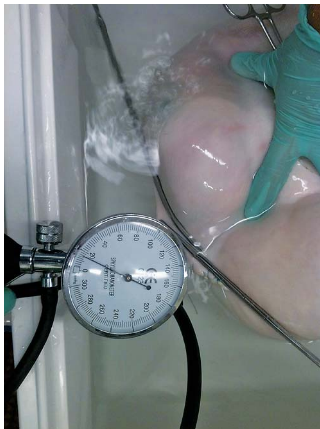
Fig. 4 Air-leak measurement procedure with the manometer and the two needles.
