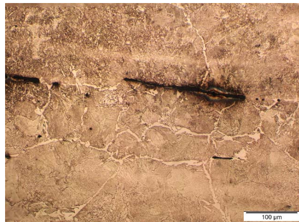
29 71306 SJM32: 2 spade (the transition from the second to the third layers) Upper: pearlite. Lower: pearlite and grid-like ferrite
