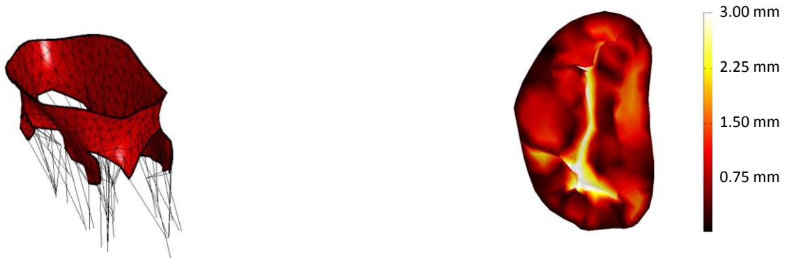
Figure 4: Simulation error for the third porcine heart simulated from the open state to closure. Color indicates error, defined as simulated leaflet distance from the leaflet shape in the experimental image of the closed valve.
