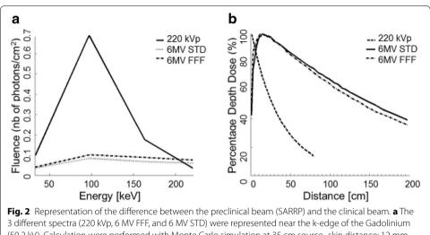
(50.2 kV). Calculation were performed with Monte Carlo simulation at 35 cm source–skin distance; 12 mm circular field size for the 220 kVp machine, and at 90 cm source–skin distance; 10 cm depth;  $10 \times 10 \text{ cm}^2$  field size for the 6 MV irradiations. **b** Percentage depth dose (PDD) for the 3 photon beams. The maximum dose for the 220 kVp occurs at the surface while it is at approximately 1.5 cm for both 6MV beams
