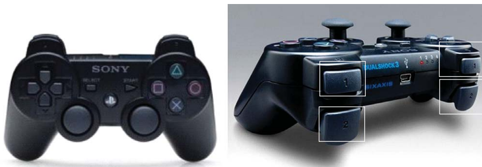
Fig. 2. PS3 ® Controller. When compared to previous controller, the PS3 ® Controller added a second pair of shoulder buttons for the middle finger in the basic button configuration. The squares indicate two pairs of shoulder buttons.
