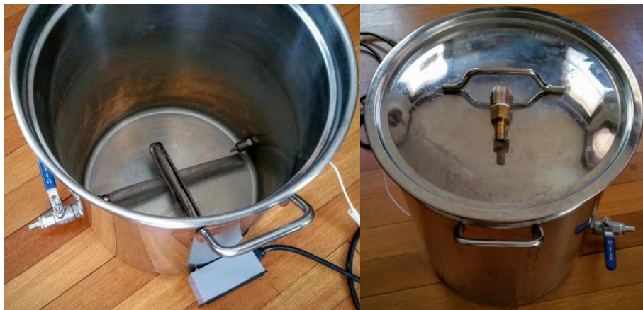
Figure 7 - Kettle with thermometer, ball valve, and heating element installed alongside cover with pump connector installed
