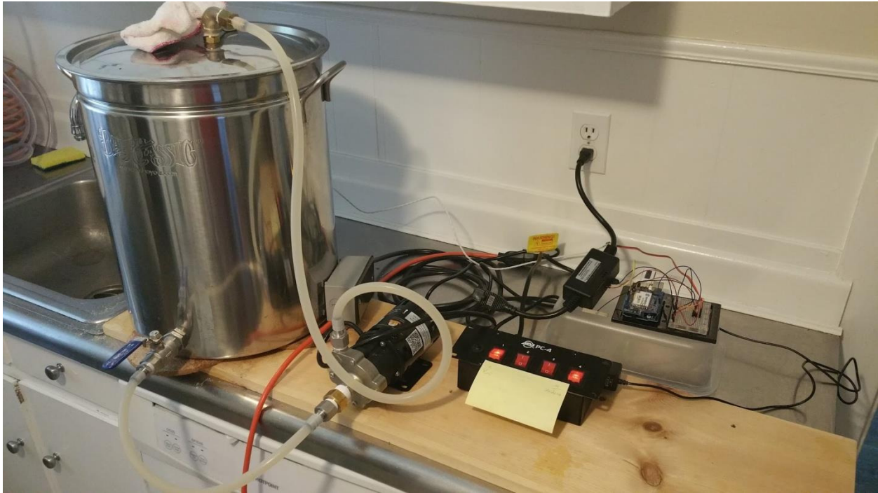
Figure 12 - Completed brewing system
