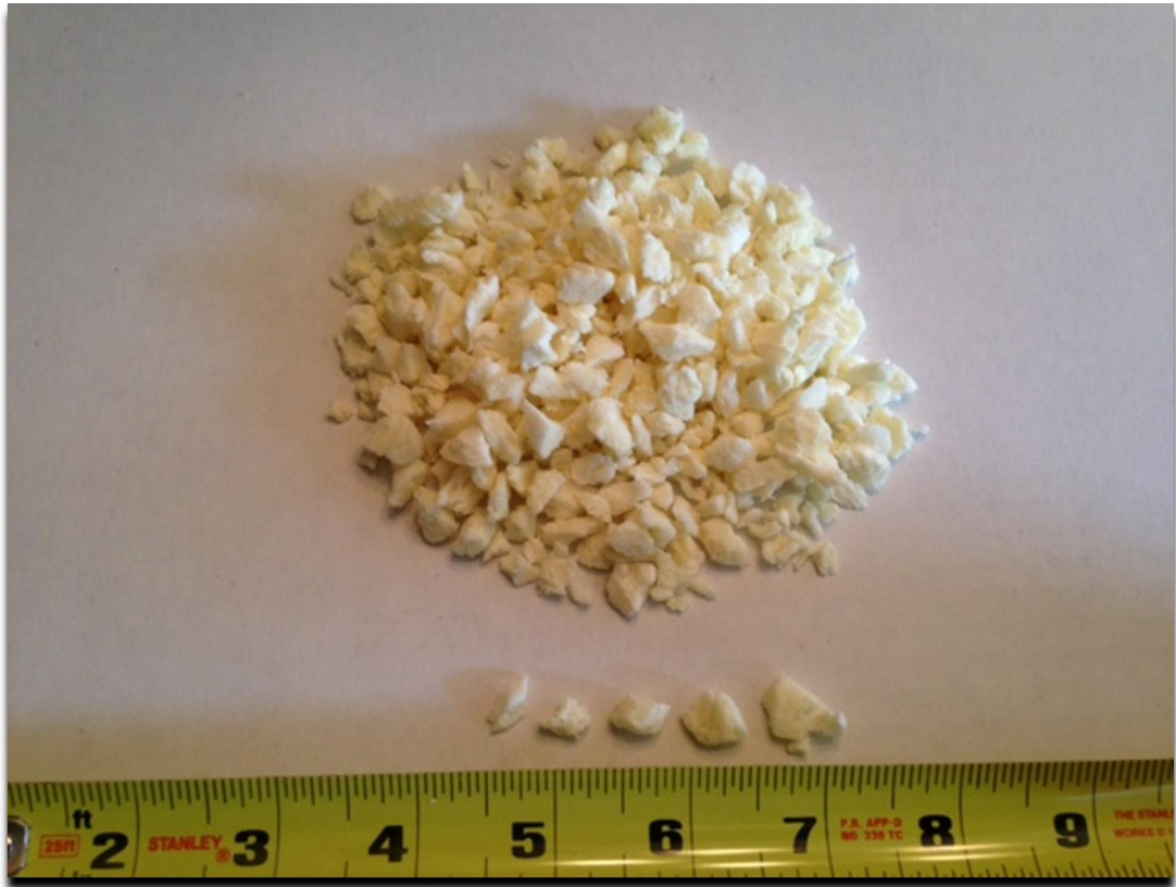
Figure 10 Appendix A. Photograph of shredded polyurethane. This figure presents a photograph of the harvested polyurethane insulation shredded into particles for Recycling Method C.
