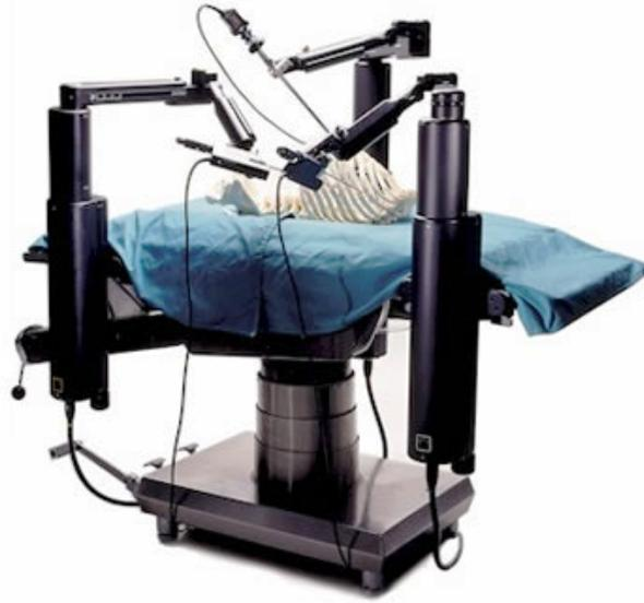
Figure 1: The Zeus Surgical Robot System.
