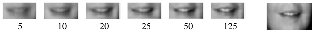
FIGURE 33. Mouth Reconstructions Varying the Number of Vectors. These reconstructions show the image quality achieved using the first 5, 10, 20, 25, 50, and 125 of the mouth vectors. The original is at far right.
