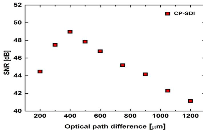
**Figure 5. Change in SNR with length of the PM fiber.** Dependence of the signal-to-noise ratio of the THz electric field measurements on the optical path difference between the two signals at the exit end of the optical fiber in the CP-SDI technique.
