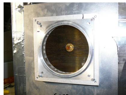
Figure 10. Another calibration source used on top of a mast for measuring \epsilon and \psi . The broadband noise source at 100 or 150 GHz outputs power through the rectangular feedhorn oriented for either vertical or horizontal polarization and through a precisely aligned wire grid to minimize cross-polarized signal.
