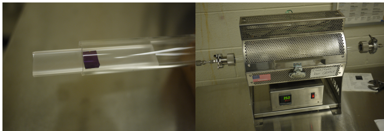
(a) Sample on a quartz boat before load (b) Image of the furnace with sample loaded inside the quartz tube.
