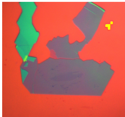
(c) The bottom stack of the heterostructure that consists of graphene (dark region in the middle) and h-BN substrate. (d) h-BN-graphene-h-BN heterostructure after completion
