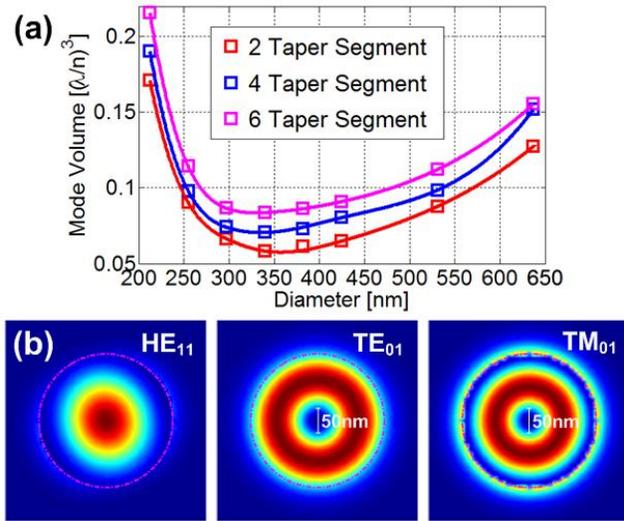
Fig. 3. (a) Mode volume as a function of micropillar diameter. Here all the modes are first-order  $\text{HE}_{11}$  modes resonating at 637nm. (b) Lateral electric field density profiles of  $\text{HE}_{11}$  ( $\lambda=637\text{nm}$ ),  $\text{TE}_{01}$  ( $\lambda=578\text{nm}$ ) and  $\text{TM}_{01}$  ( $\lambda=492\text{nm}$ ) cavity modes.
