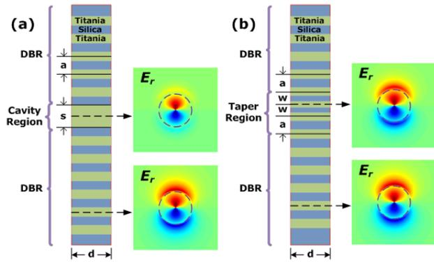
Fig. 1. (a) Traditional design of micropillar cavities and (b) modified design where the center segment is substituted by titania/silica pairs. The lateral mode profile of  $E_r$  component for cavity mode and evanescent Bloch mode that exists inside DBRs are shown on the right of the cavity layout. Improved mode-matching can be seen in (b).
